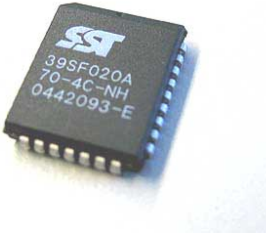
BIOS chip for VIA M10000 mainboard
